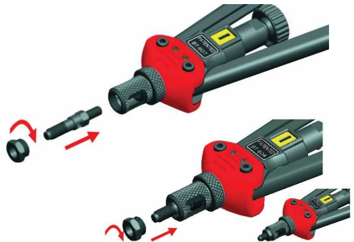
Figure F. To release mandrel, push the inner sheath back and unscrew the mandrel.
