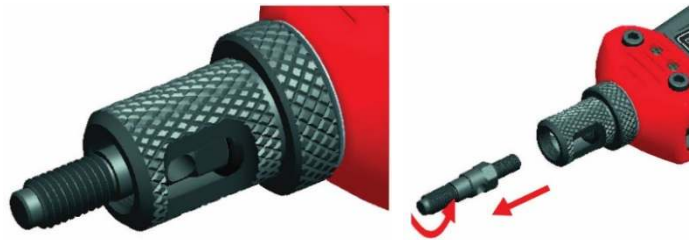
Figure F. To release mandrel, push the inner sheath back and unscrew the mandrel.
